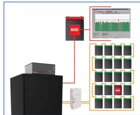
Battery Monitoring Identifies Bad Cell
