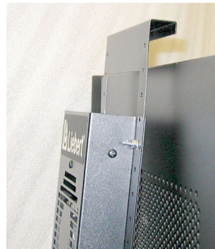
XDA with mounting bracket being hung on door
