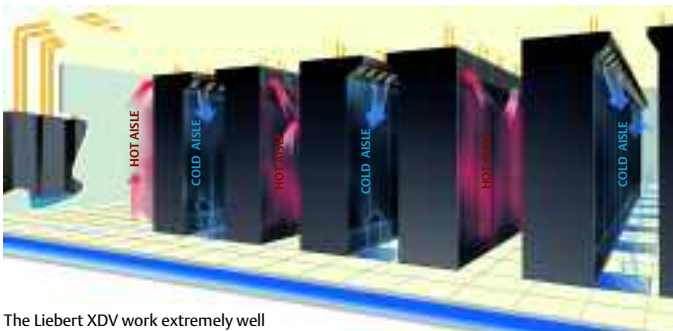
The Liebert XDV work extremely well with the "hot aisle-cold aisle" approach.
